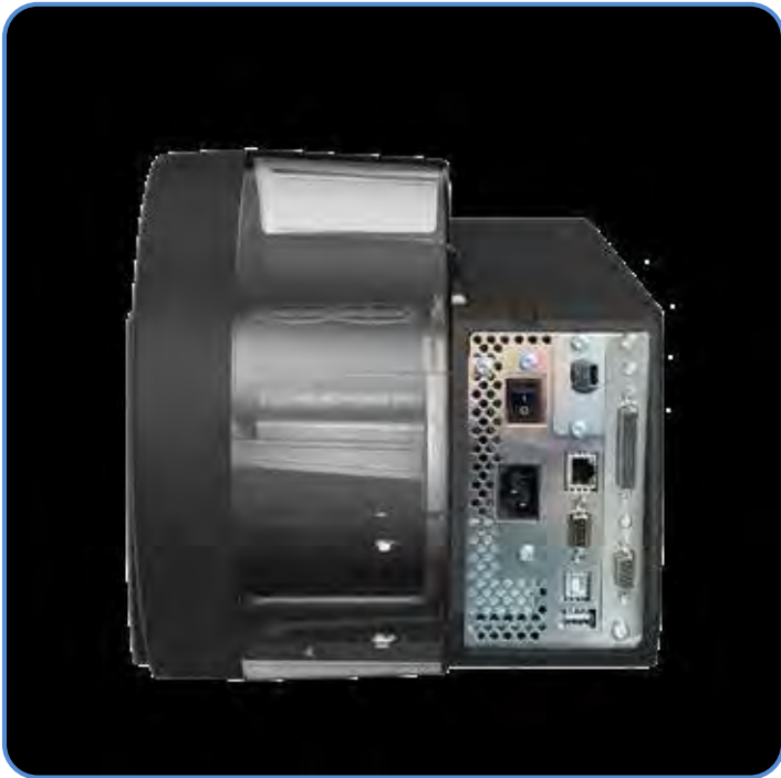
PM45C has 1 x I/O Expansion Slot
