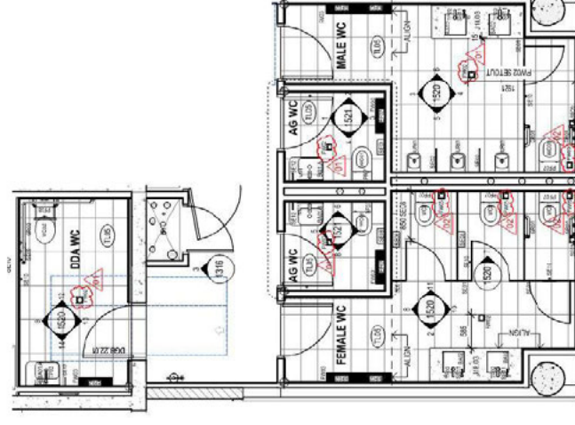
Typical All Gender Layout – Pod B with bank of Female/Male and Unisex Accessible Toilets
