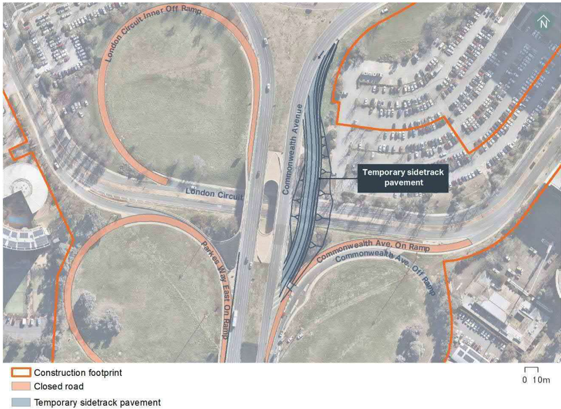
Figure 2-3 Temporary Commonwealth Avenue sidetrack configuration
