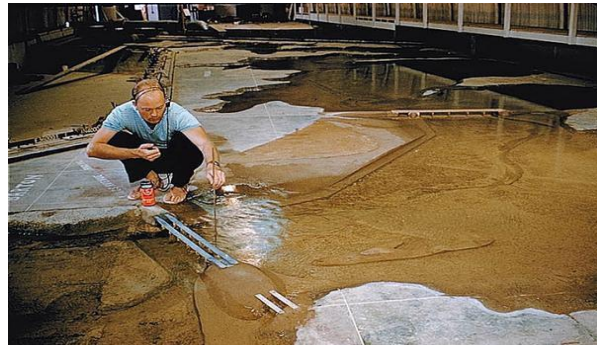
Figure 2.9 Flow measurement at Kings Ave Bridge, with Central Basin and Commonwealth Ave Bridge. (Source: National Library of Australia, nla.obj-143692313)
