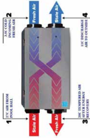
Figure 21 Typical heat exchange process on a 3.5C cold day.
