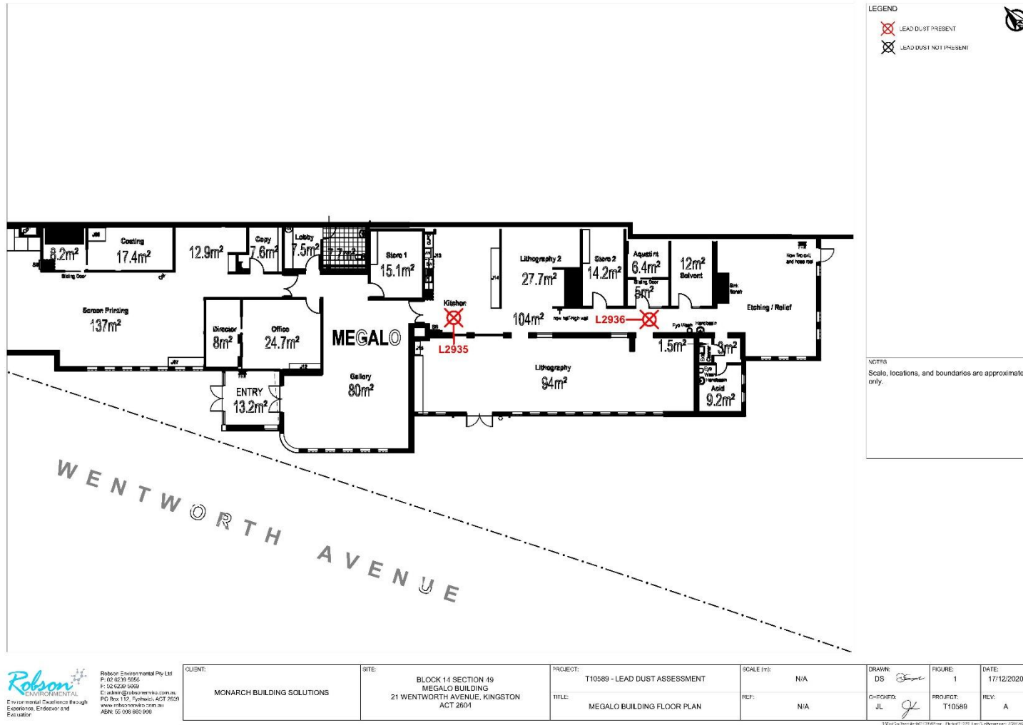
Figure 3: Location of lead dust swab samples in the Megalo Building at the Old Bus Depot Markets
