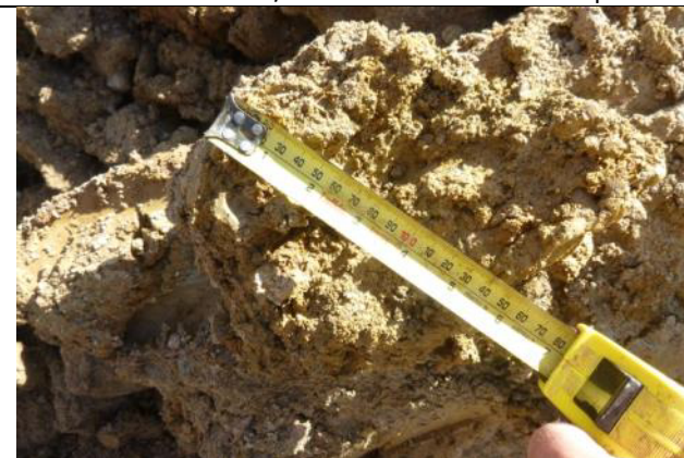
Test Pit T05 – Zone 1 Silty CLAY core material spoil
