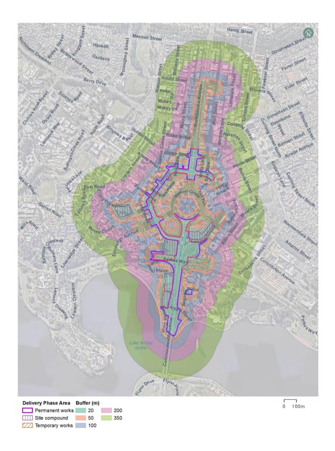
Figure 15-1 **Buffer distances for Construction Footprint**
