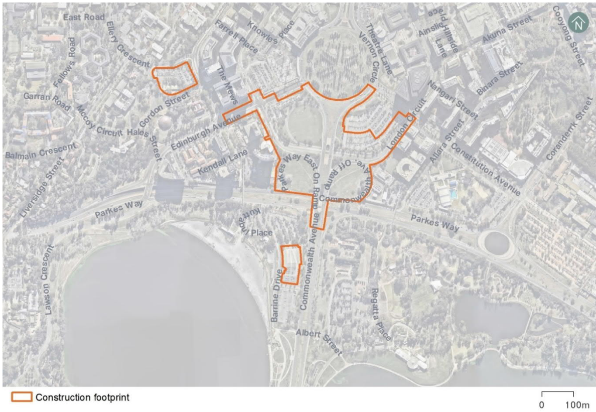
Figure 2-2 The Project construction footprint and early works areas
