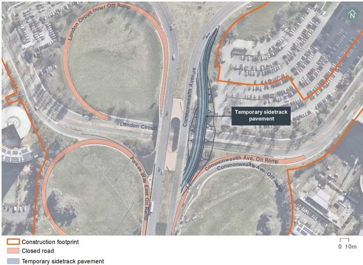
Figure 2-3 Temporary Commonwealth Avenue sidetrack configuration
