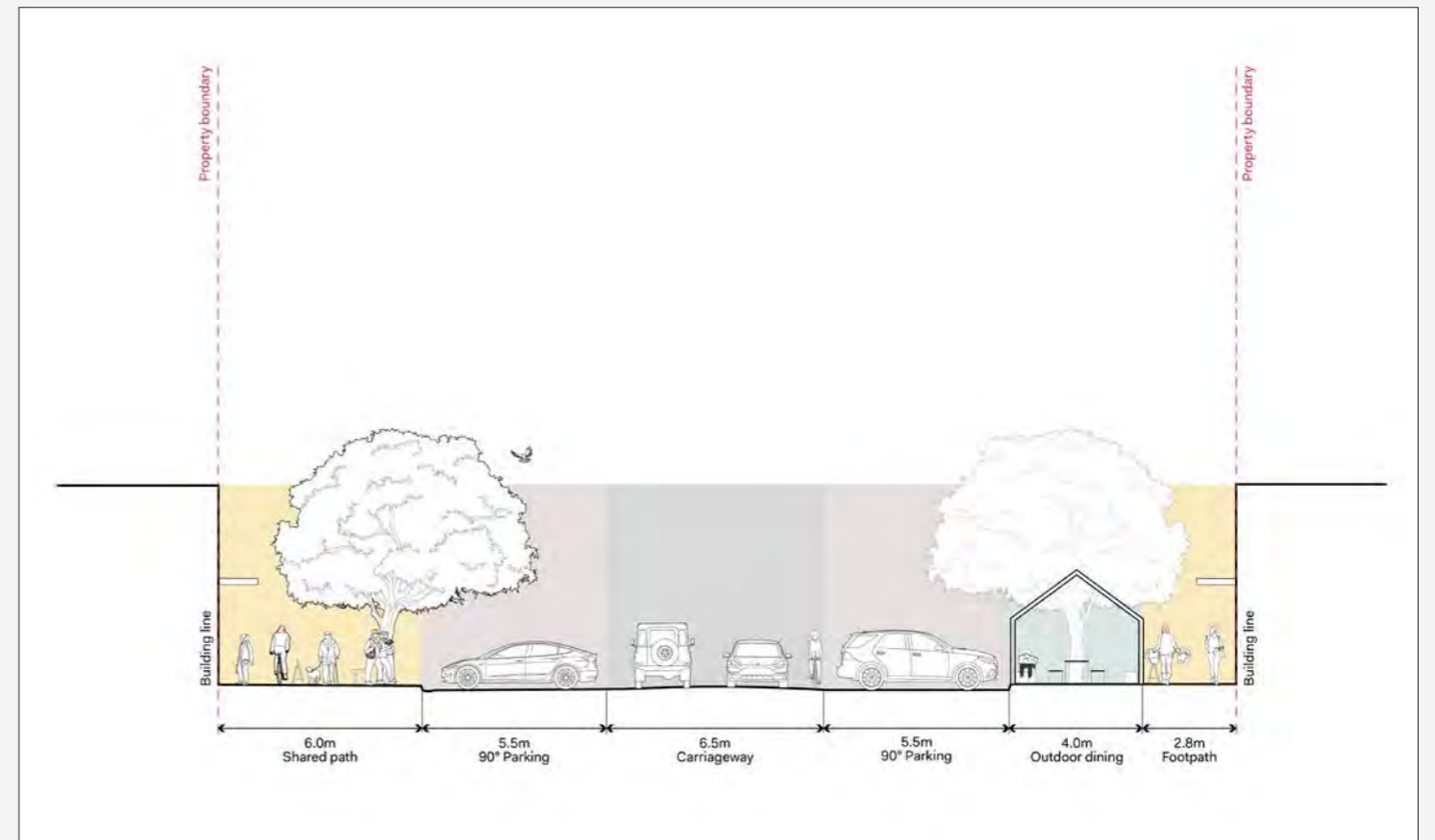
Existing | Woolley Street | North-South Typical Section
