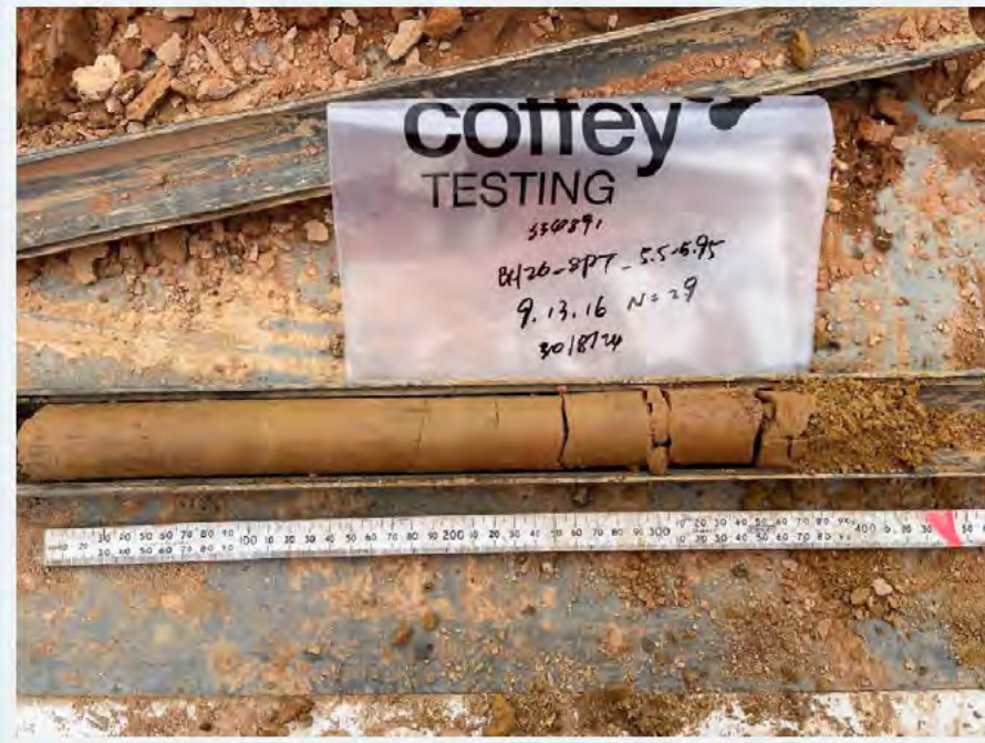
Photo 14 – SPT sample from BH26 at depth between 5.5 – 5.95m bgl.
