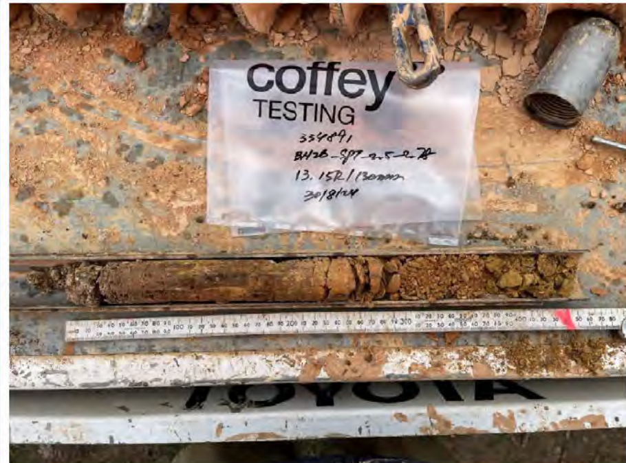
Photo 12 – SPT sample from BH26 at depth between 2.5 – 2.78m bgl.
