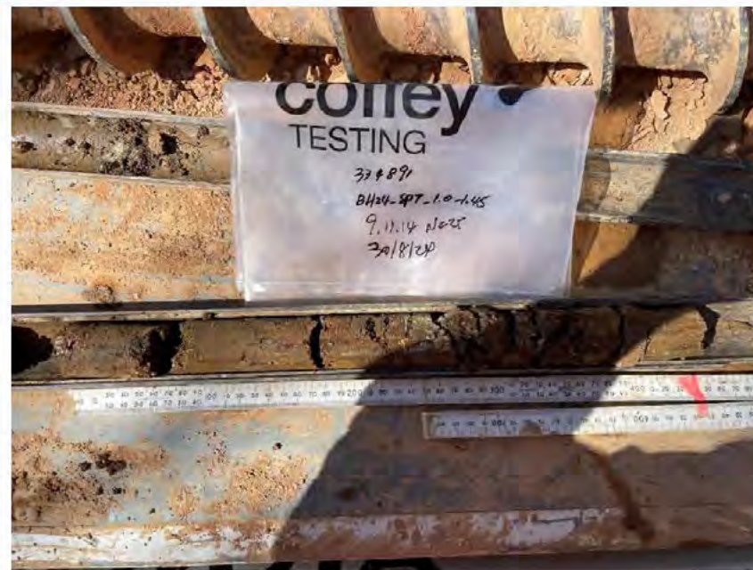
Photo 8 – SPT sample from BH24 at depth between 1.0 – 1.45m bgl.
