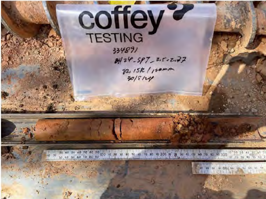
Photo 9 – SPT sample from BH24 at depth between 2.5 – 2.77m bgl
