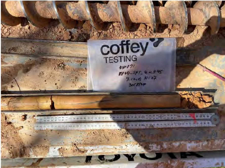
Photo 10 – SPT sample from BH24 at depth between 4.0 – 4.45m bgl
