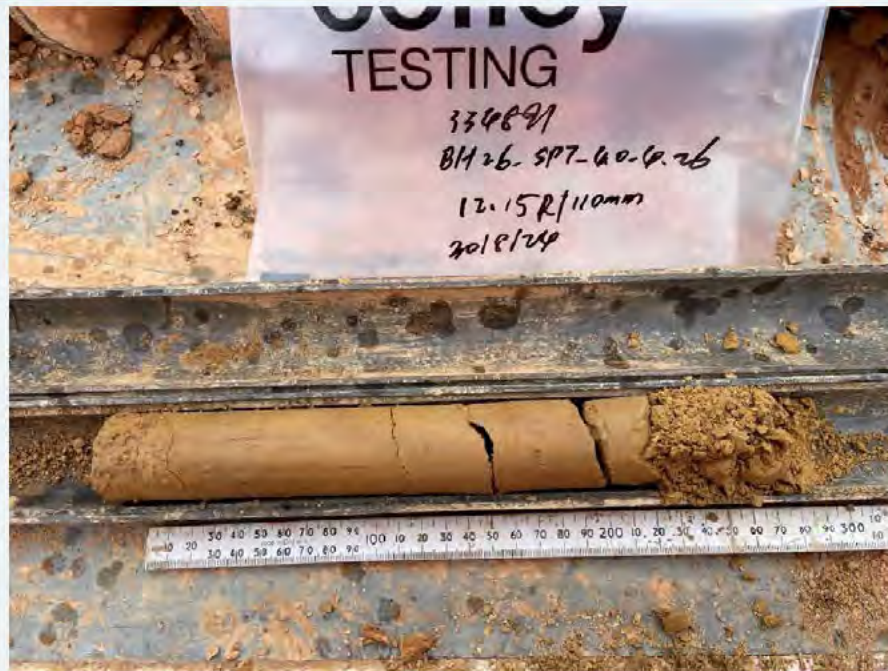
Photo 13 – SPT sample from BH26 at depth between 4.0 – 4.26m bgl.
