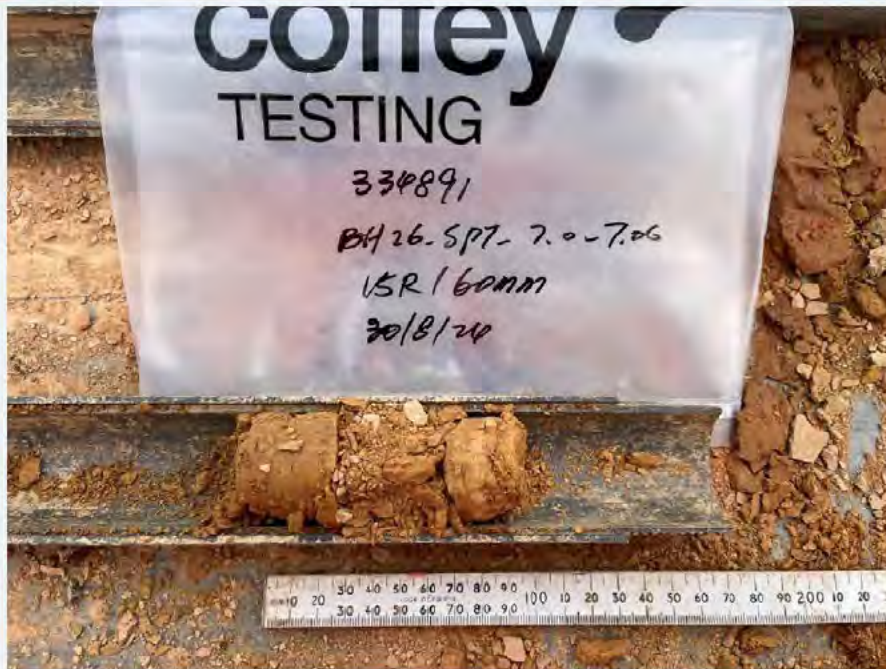
Photo 15 – SPT sample from BH26 at depth between 7.0 – 7.06m bgl.
