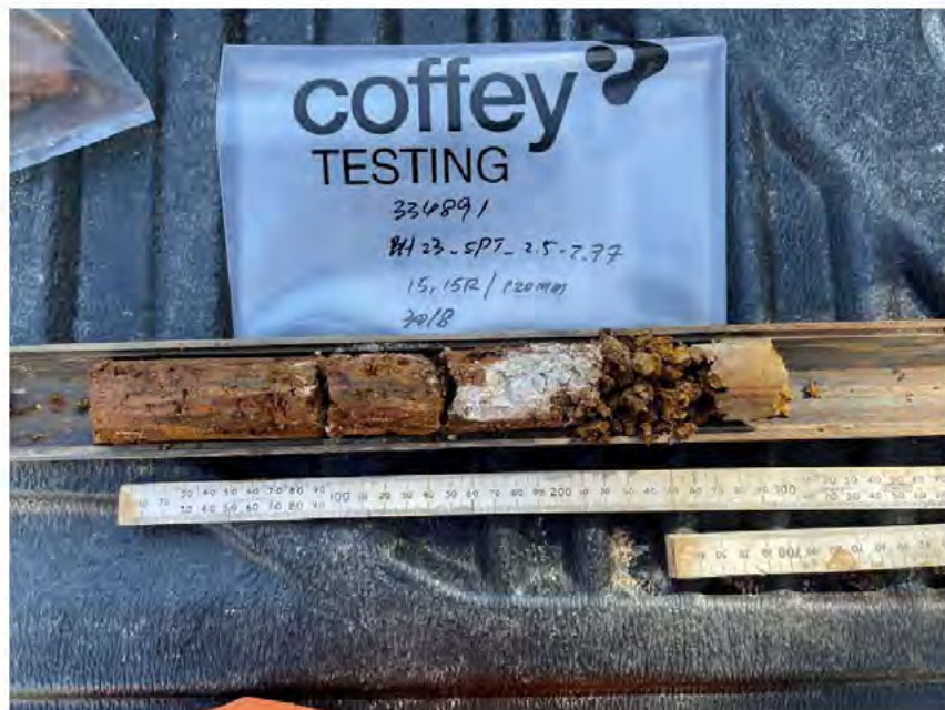
Photo 7 – SPT sample from BH23 at depth between 2.5 – 2.77m bgl.
