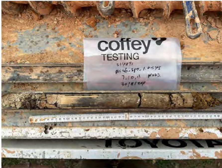
Photo 11 – SPT sample from BH26 at depth between 1.0 – 1.45m bgl.
