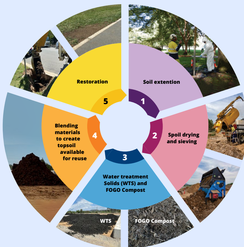
Figure 8 Icon Water’s Spoil to Topsoil project process
