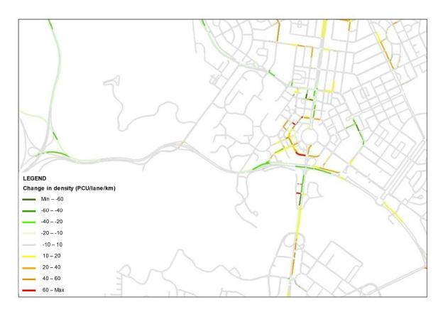
Figure 7-14 Network density changes with the Project compared to without the Project during the weekday AM peak hour in 2036
