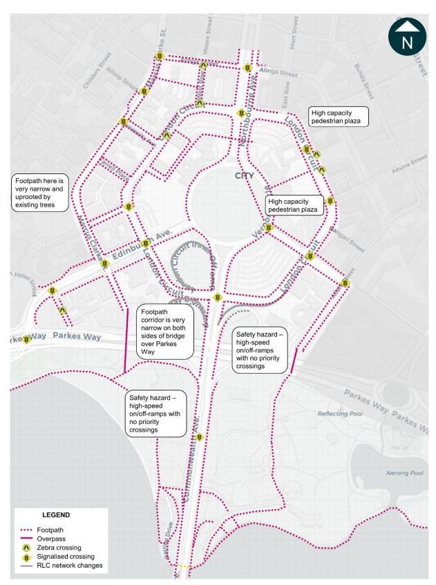
Figure 5-18 Existing pedestrian infrastructure (including planned changes due to RLC)
