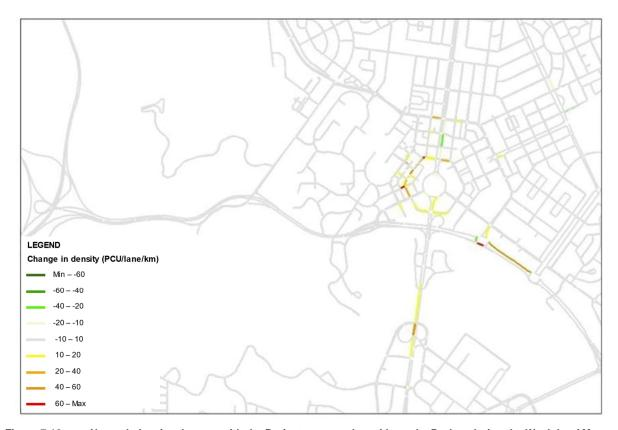
Figure 7-12 Network density changes with the Project compared to without the Project during the Weekday AM peak hour in 2026
