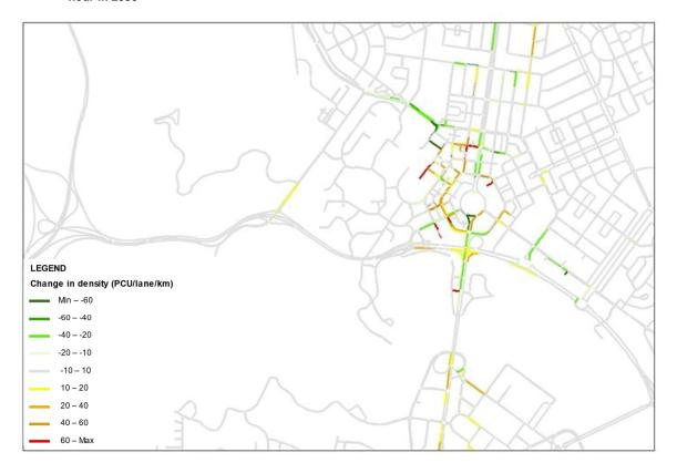
Figure 7-15 Network density changes with the Project compared to without the Project during the weekday PM peak hour in 2036
