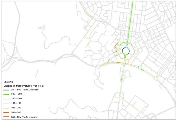
Figure 7-4 Traffic volume changes with the Project compared to without the Project during the weekday AM peak hour in 2026
