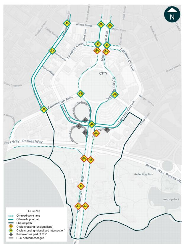
Figure 5-19 Existing cycling infrastructure (including planned changes due to RLC)
