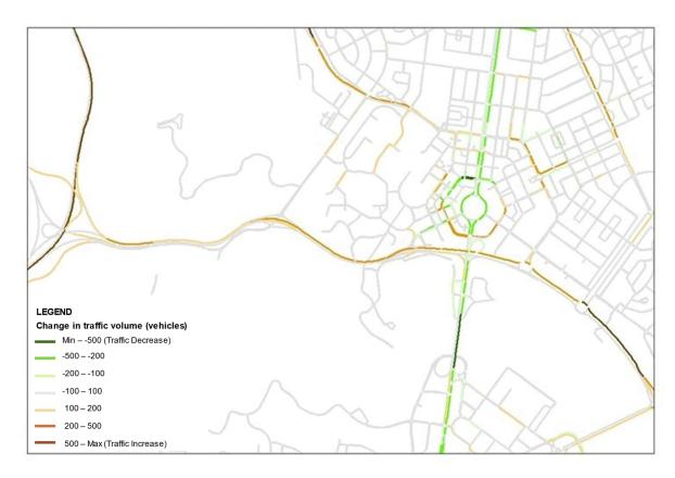
Figure 7-6 Traffic volume changes with the Project compared to without the Project during the weekday AM peak hour in 2036
