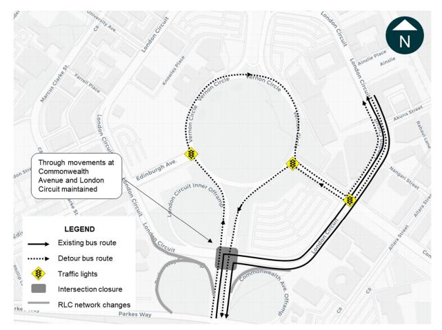
Figure 6-6 Commonwealth Avenue and London Circuit proposed bus diversions
