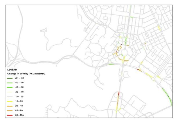
Figure 7-13 Network density changes with the Project compared to without the Project during the Weekday PM peak hour in 2026
