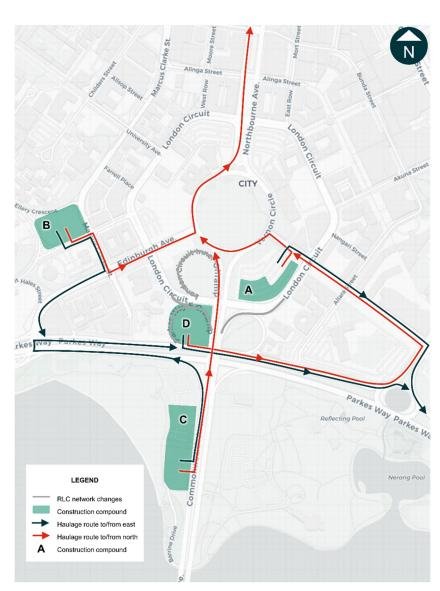
Figure 6-4 Outbound haulage routes from construction compounds
